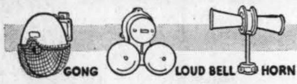
Some locations are so noisy the ordinary telephone bell cannot be heard. In such cases a gong. loud bell or horn is needed. Where there are several telephones at one location, they can be fitted
